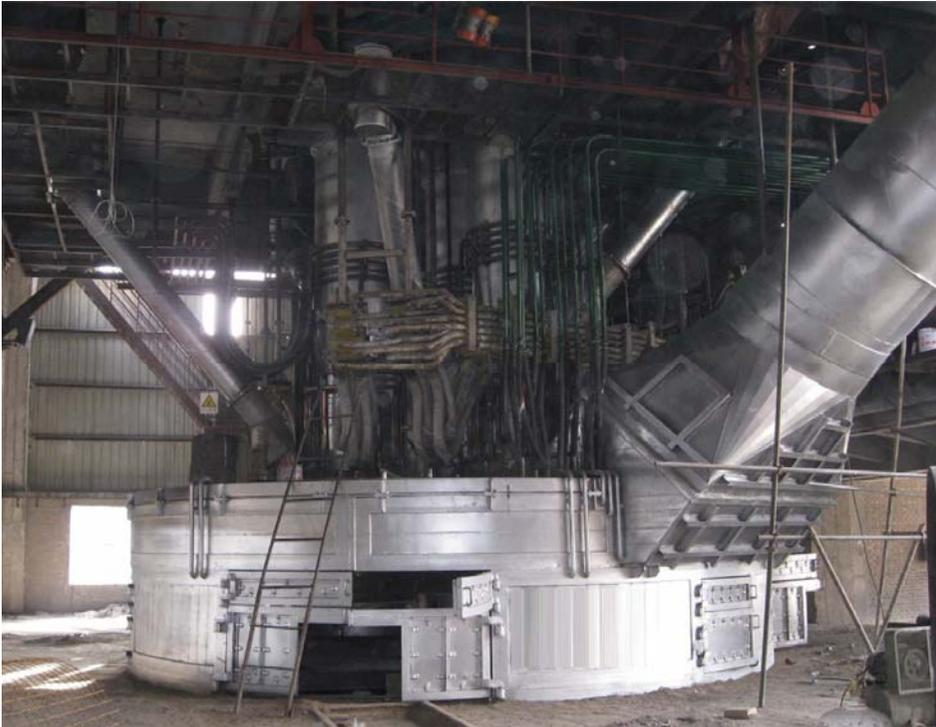
Ferroalloy Submerged Arc Furnace
