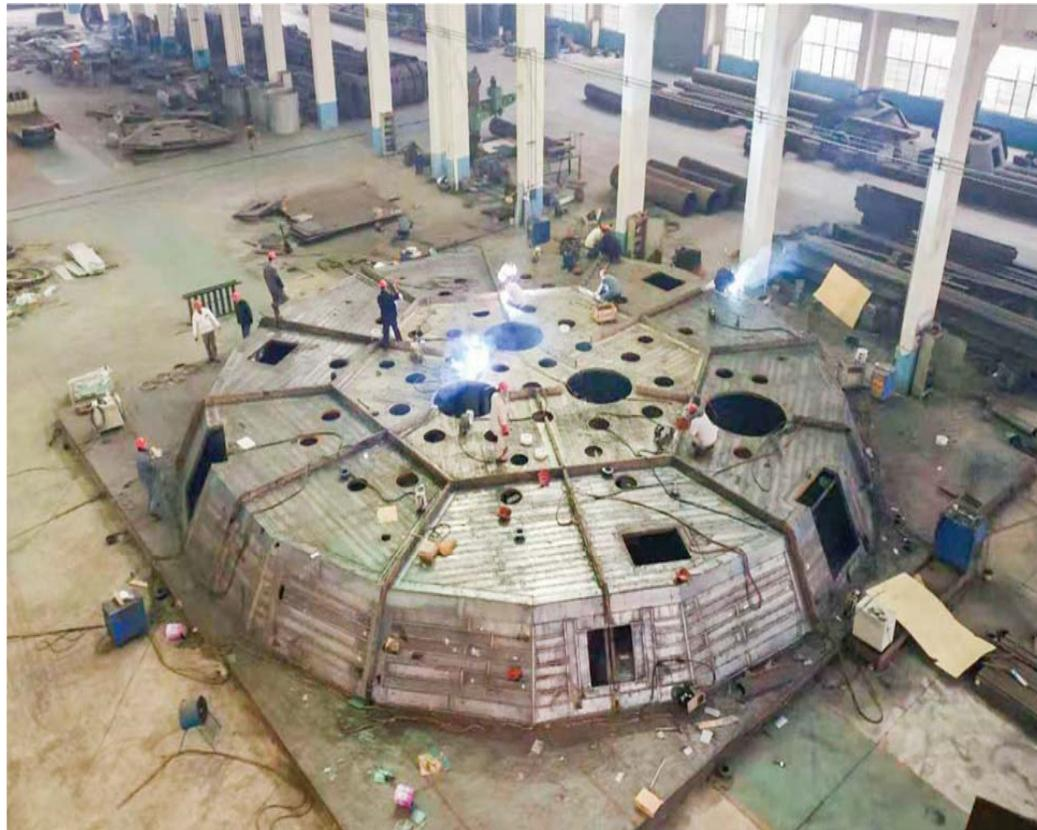
Manufacture and Assembly of Large Airtight Submerged Arc Furnace Cover Factory
