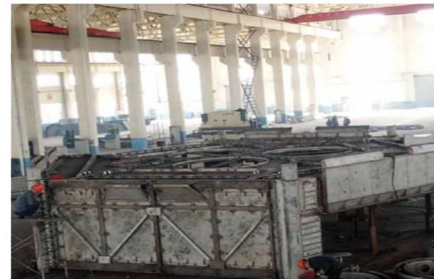
Large all stainless steel semi-closed furnace cover factory production and assembly
